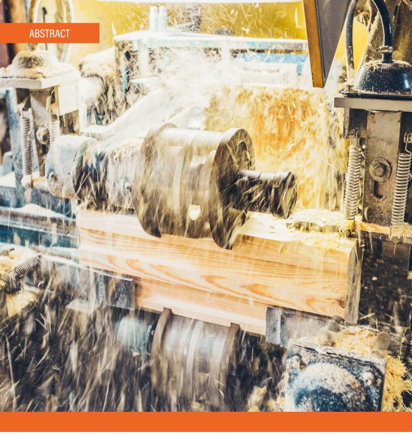
There are two common methods that can be implemented to subdue a dust explosion isolation and suppression. Isolation prevents the propagation of the flame, pressure, and ignition of dust cloud in a secondary enclosure. Suppression is a method that detects and eliminates an explosion in the early stages of development.
